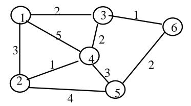
(i) Use the Dijkstra's algorithm to find the set of shortest path from node 2 to other nodes.
