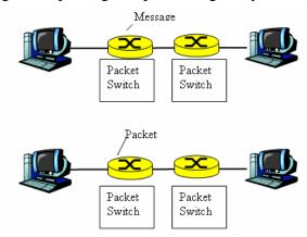
a. Consider sending the message from source to destination without message segmentation. How long does it take to move the message from source host to first packet switch? Keeping in mind that each uses store-and-forward packet switching, what is the total time to move the message from source host to destination host?
